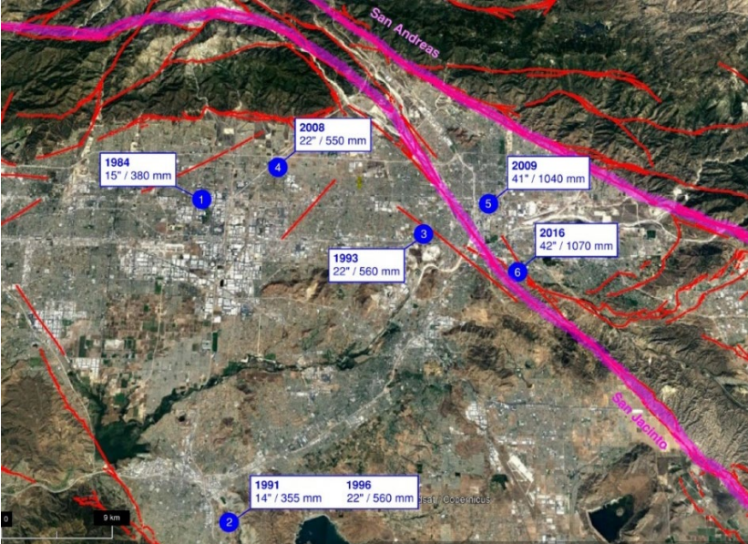
Figure 10 Maximum design displacements for seismically-isolated buildings in inland southern California, 1984-2016. (image: adapted from Google Earth).
