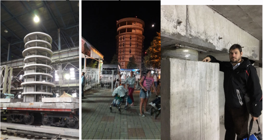
Figure 18 Anapa airport control towers testing model and real building (LRB)
