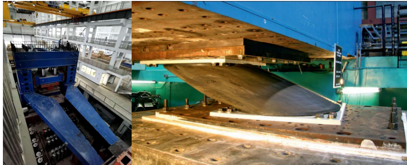
Figure 6 10000-ton tri-axial testing system for seismic isolator and damper
